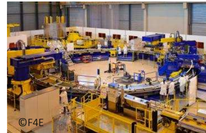
ITER - PF Coils manufacturing
