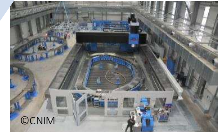
ITER – 35 Radial plates manufacturing
